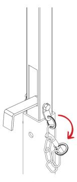
3. Rotate rapid pin into locked position.
