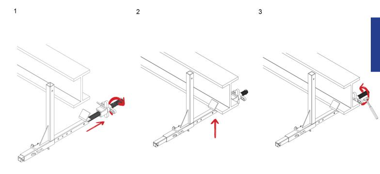
1. Extend the clamp so that it has sufficient clearance to fit around the flange of the beam. 2. Position the clamp on the beam.
