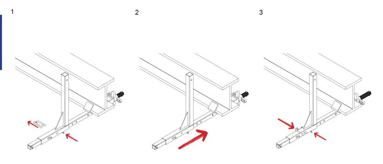
1. Remove the Rapid Pin from the arm and loosen the sliding thumb screw from the underside of the clamp.
