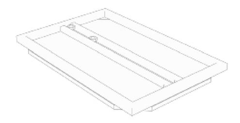
IMPORTANT: PRODUCT REQUIRES MINIMUM 2NO. 25KG / 55LBS BALLASTS TO BE PLACED ON EACH FOOT TO CONFORM WITH BS EN13374:2013+A1:2018 AND MINIMUM 3NO. 25KG / 55LBS BALLASTS TO BE PLACED ON EACH FOOT TO CONFORM WITH OSHA 1926.502
