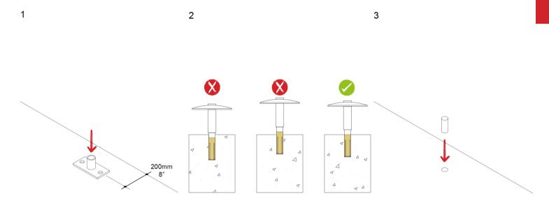
1. Using the drill alignment tool, drill a hole to accept an ØM16mm x 50mm / Ø5/8" x 2" wedge anchor, to manufacturers specification. 2. Check hole is the correct depth.
