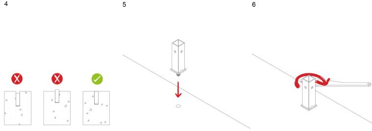
4. Check anchor bolt fits correctly into the drilled hole. 5. Screw socket base into wedge anchor.
