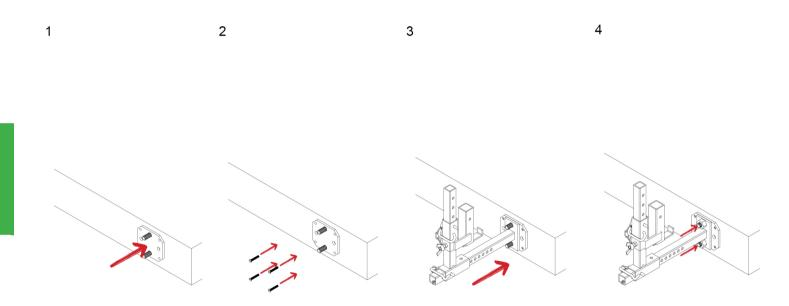
1. Hold Adapter Face Plate in place against CLT edge.
