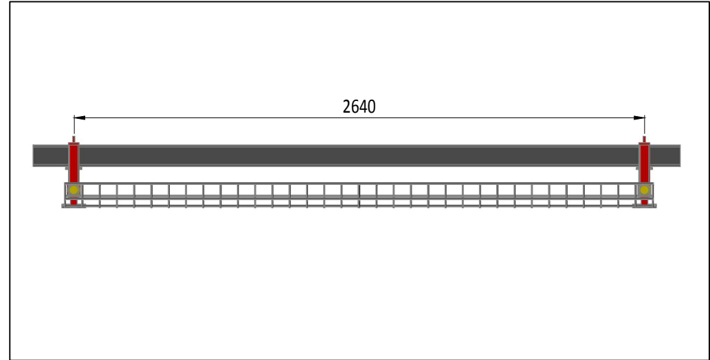
CLAMP PLACEMENT: ENSURE THAT THE BOX CLAMPS ARE SET AT MAXIMUM CENTERS OF 2640mm
